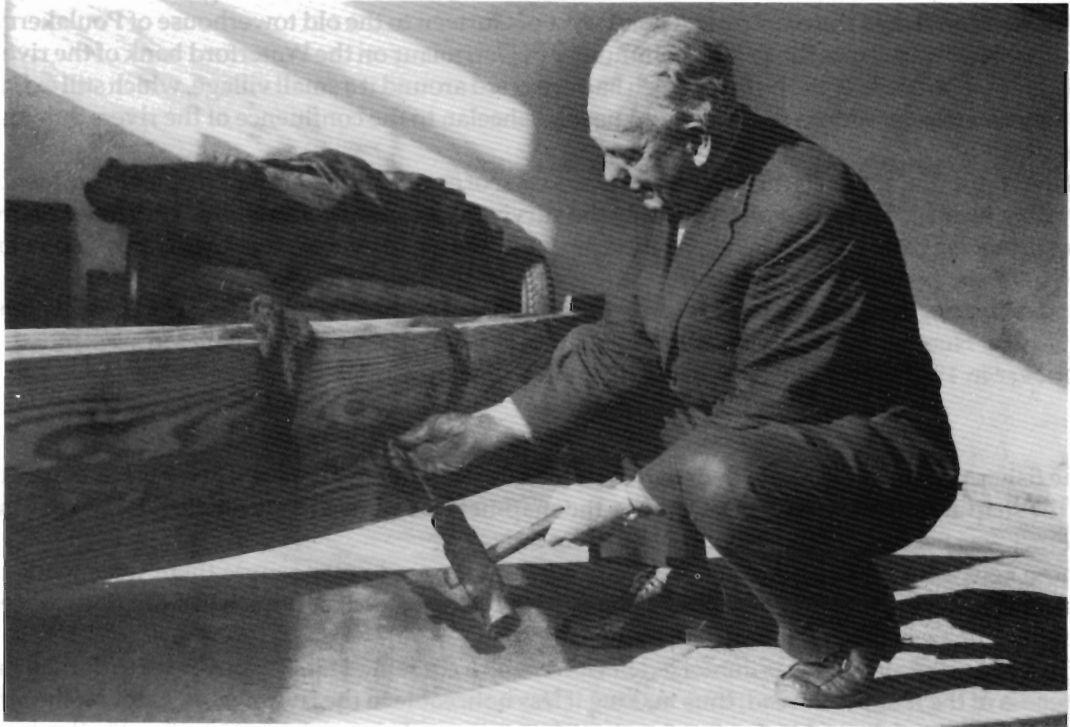
Caulking iron and hammer being used by Michael O'Callaghan, who learned the skill at Kehoe's graving dock in Carrickbeg early in this century.
