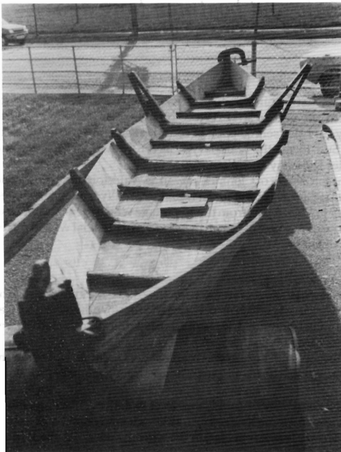
Old-style cot under construction by Michael O'Callaghan. Note that he has fitted boards between the timbers to further strengthen the floor of the cot.
